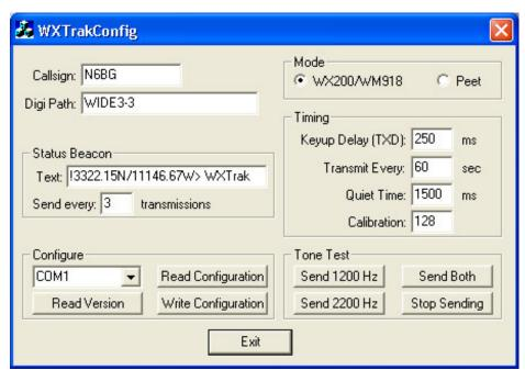
Reading the Configuration is always performed twice and compared in the program to insure correct data. Writing the configuration is always followed by a read and compared to insure correct data. A dialog will notify the user when the read or write is complete, and if it was successful. A read or write operation may fail if the unit is transmitting. If this happens, simply try again. Detailed information about each configuration parameter is included below.
