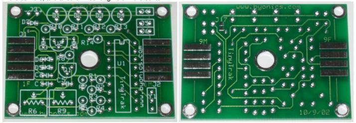
If desired, 0.15 inch can be cut or sheared off each end of the PCB to allow an alternate case fitting.
